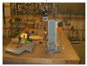
We had to make a few changes along the way to allow the using of lead screws that were milled down to allow for ½ "bearings on each end. With a 24" lead screw length, we ended up with a little over 21" of cutting area on the Y axis. This was
