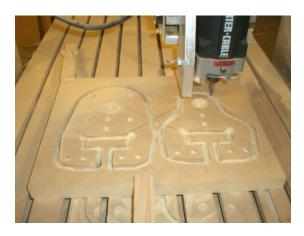
The larger pieces had to be hand made due to the limited cutting area of our existing machine. We used the stepper motors and controller from the first machine on the new one. We added another axis driver to the controller to support the dual stepper motors on the X axis. All the special parts; lead screws, v-groove bearing, and couplers were purchased on line from various suppliers. All the other items were purchased locally from building and hardware suppliers.
